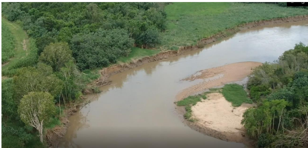
Figure 81. The downstream section of Murray Creek case study area within the estuary where the banks consist of estuarine muds and there are sandy instream deposits.
