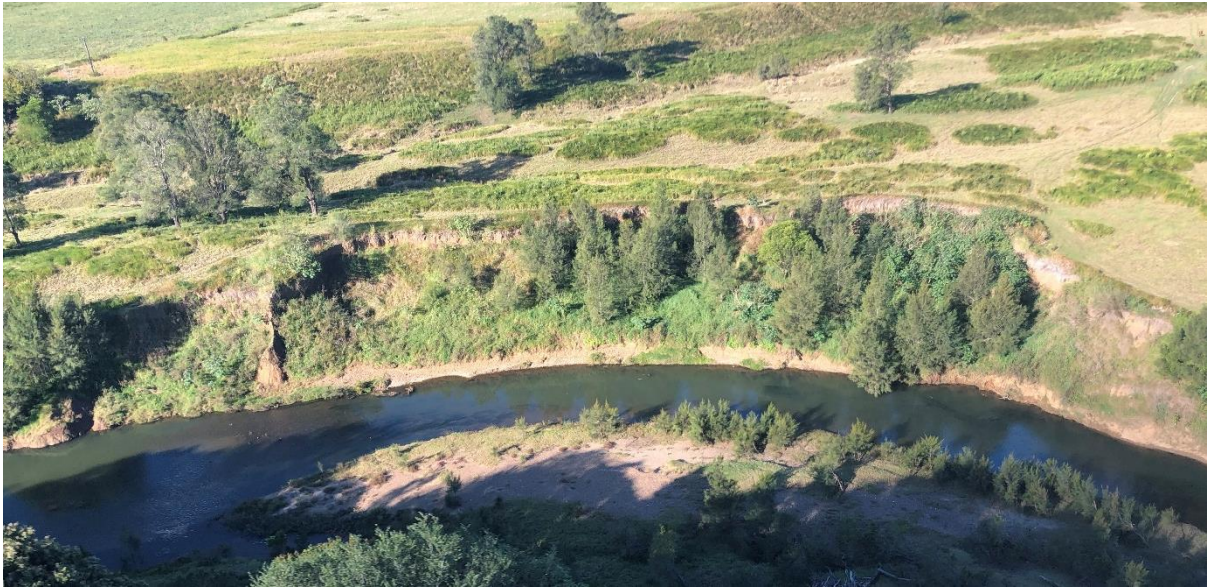
Figure 15: Meander development within an inset floodplain near Ashton Road within the Mary River case study area
